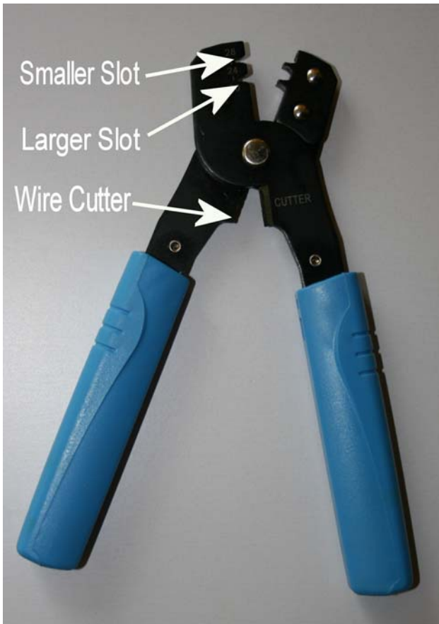
The Crimping Tool showing the smaller slot (marked 24 - 28), the larger slot (marked 20 - 24) and the wire cutter
