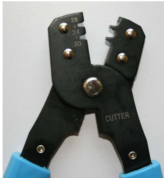
Crimping Tool head showing the slots and markings
